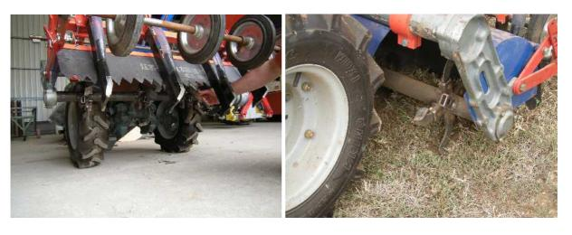
Note how Jack and Matin have made up a new axle, which holds the tiller blades. There are eight blade holders at each site, and various configurations of left hand, right hand, straight and angled blades can be fitted. Depending on the configuration used, different widths of slots can be cut, as well as various slot shapes.
